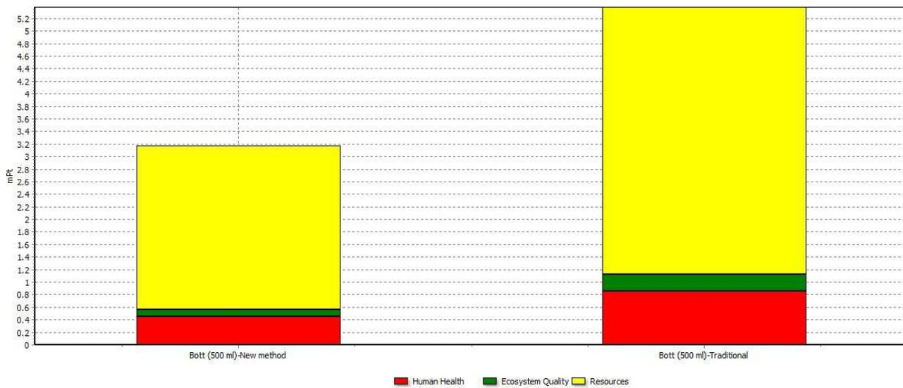
**Figure 12:** Bottle production main environmental effects. Comparison between the two different processing methodologies.
