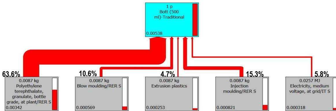
Figure 7: Process tree concerned with the bottle produced through the traditional system.
