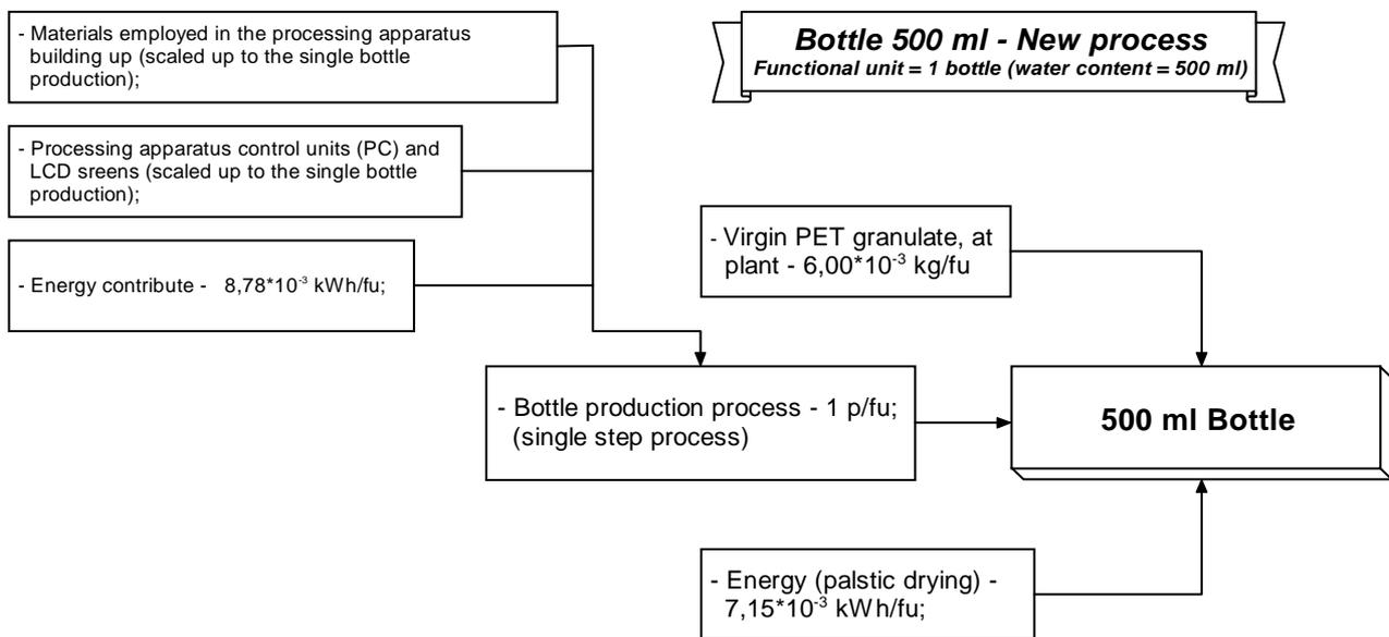
Figure 6: Flow chart of the new process employed in the bottle production.
