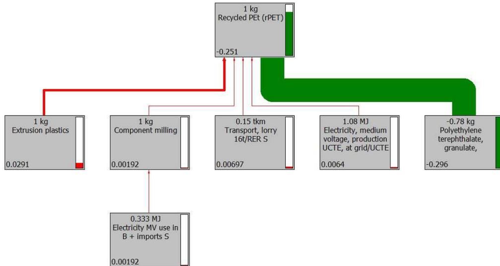
Figure 9: Process tree concerned with the PET recycling.
