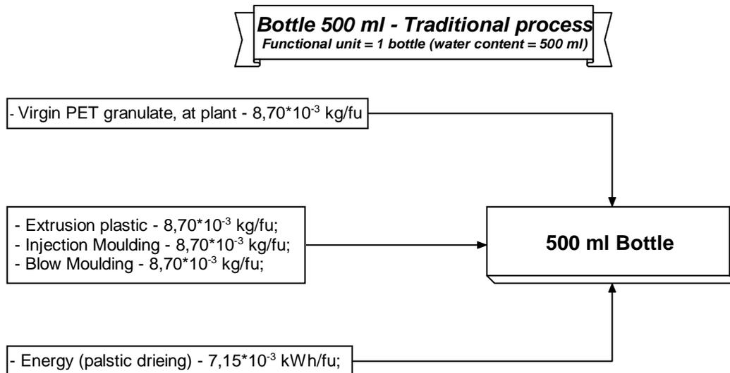
**Figure 5:** Flow chart of the processes employed in the traditional bottle production.
