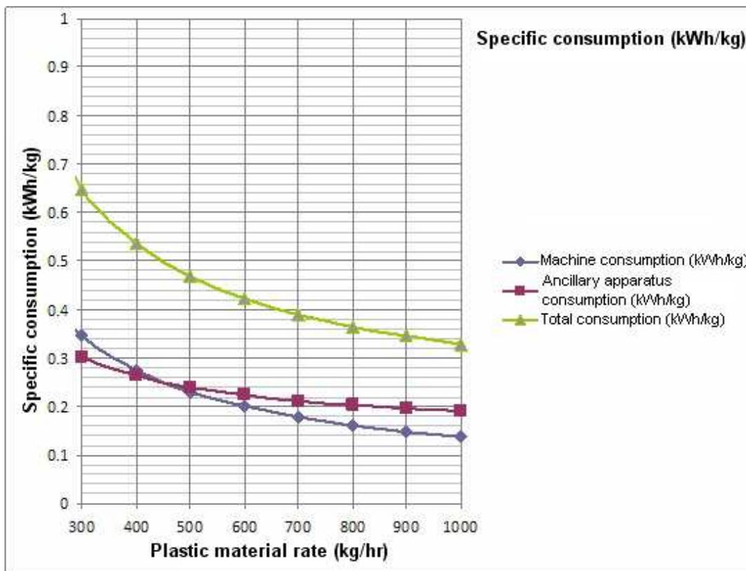
Figure 1: Energy consumption versus processed material rate.
