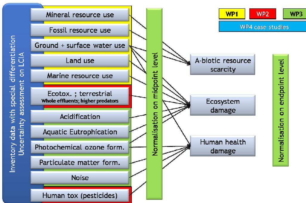
Figure 4: Schematic representation impact categories (factors) and the related effects the lead to.
